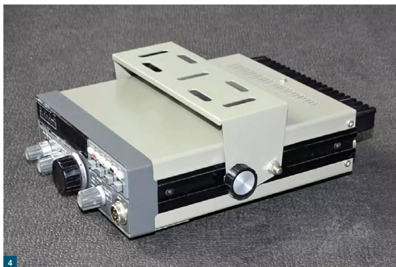
Fig. 4: The R0062900 universal mounting bracket engages the side rails of the transceivers.
